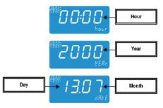
Each time the MDS controller is disconnected from battery the date and time will require adjustment. As long as battery power remains the date and time will be retained.
